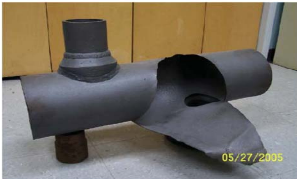
Figure 4-116 – Sulfidation failure of NPS 8 carbon steel pipe. Note the relatively uniform thinning that resulted in a sizeable rupture.
