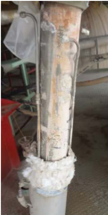
PV-9002 found with salt deposits & without inner protective oxide layer
