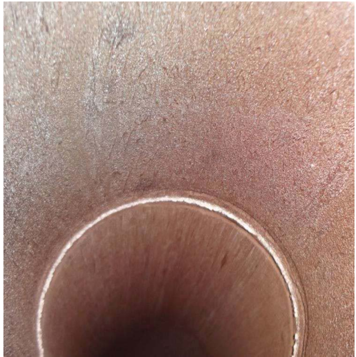
PV-9002 found with salt deposits & without inner protective oxide layer
