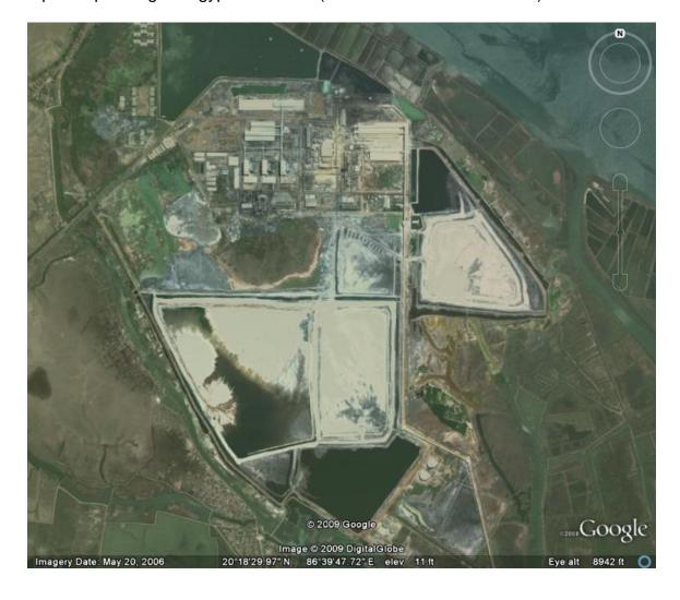
The next photo shows a plant of approximately 1MM  $P_2O_5$  t/year capacity with a gypsum stack (scale 3.2 km across bottom) in Florida, USA.
