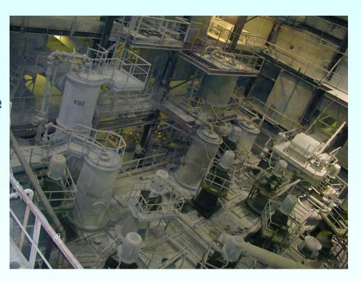
> washing of the cake with countercurrent water to obtain the return phosphoric acid with sending it back to the stage of decomposition.
