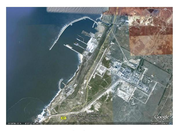
The above photo shows the Jorf Lasfar plant in Morocco that uses seawater for process cooling and for gypsum slurry transport to the ocean. The approximate scale is 8 kilometers across the bottom of the photo.
