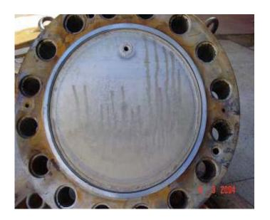
No gasphase and no condensation corrosion
