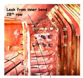
Additional tube leaks confirmed on pressurization and opening of the refractory. ( 27th & 26 row)
